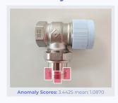
**Top Composite Image:** Normal state **Bottom Image:** Anomaly detected — missing black band
